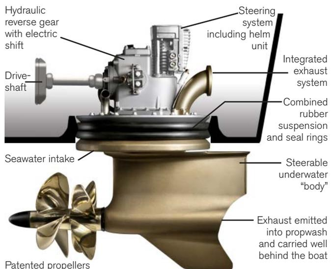
The Volvo Penta IPS has been developed and is manufactured as a complete system with everything included – engine, propulsion unit incl. gear box, propellers, exhaust and seawater system, steering, and controls.
